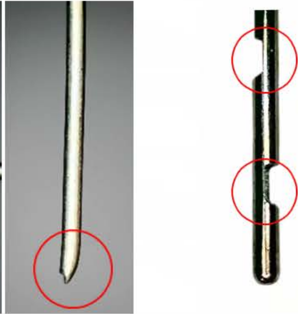
SS Irrigation Needle from other other vendors With cutting on tube wall [2]
